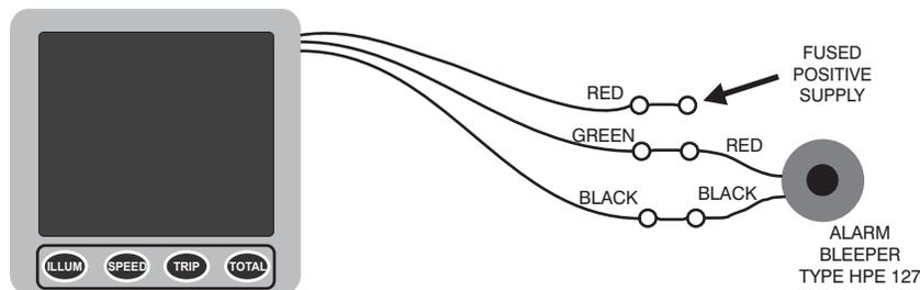
**Figure 1 - Wiring Installation**
