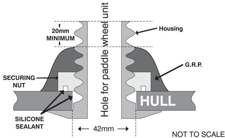
**Figure 2 - Paddle Housing Installation (Sectioned view)**
